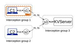
(a) A key-value store (S-KV) composed of two shards and a router.
