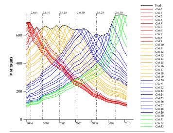
Figure 16. Lifetime of faults across versions
